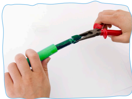
Step 2: Remove ink reservoir.
